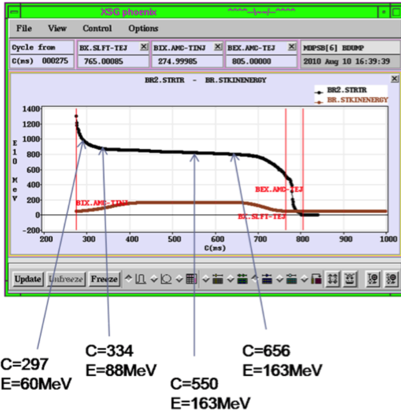
Figure 1: The kinetic energy (brown bottom curve) and the beam intensity (black top curve) are shown as a function of cycle-timing for the 160 MeV flat top cycle. The four measurement points are labelled.
